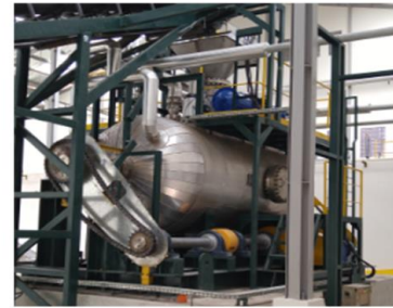
Hydrothermal Reactor: Treat MSW with high pressure/temperature steam
